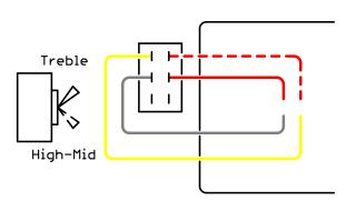
\*Wired as shown, inserting 1/4" mono cable into stereo jack will apply power to U2B. Remove cable when not in use to preserve battery life.
