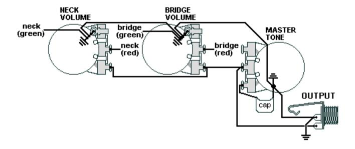
For each pickup, solder the black&white wires together and tape up each connection.
