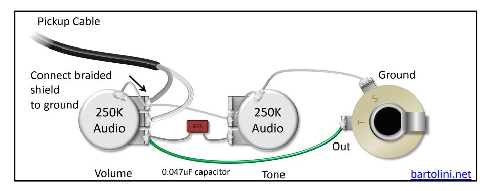
The diagram below is a very simple setup for passive tone and volumes for two pickups using 1-conductor cable.
