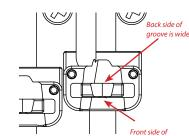
The insert groove has a slight downward angle for string relief. When installed correctly, the saddle groove should flare out in the back (as shown).
