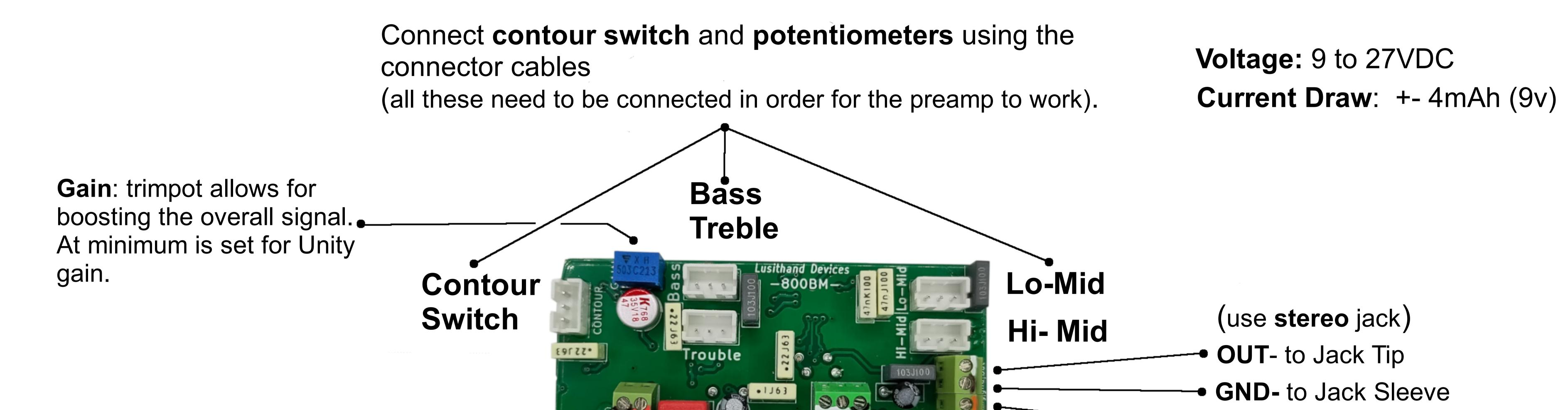
Black: - battery black wire-\_\_\_\_\_ Red: + battery red wire-\_\_\_\_\_
