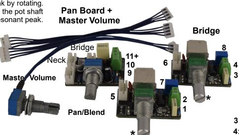
7/8: These trimpots act as attenuators for hotter pickups that sound louder or create clipping on the preamps input. It shipps set to 0 attenuation.
