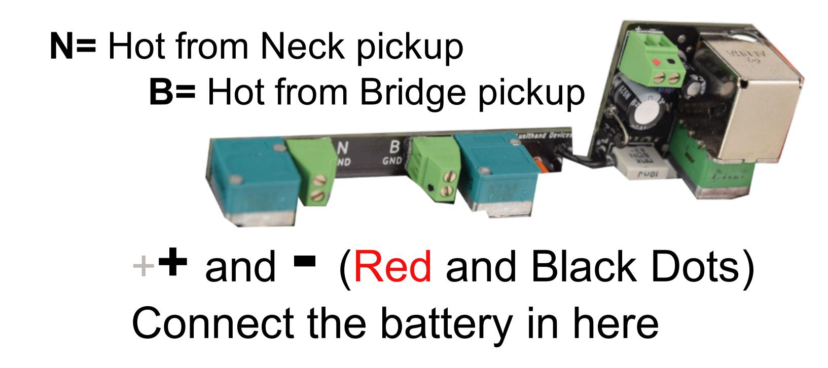
**GND x2=** Ground wires from pickups(usually black) connect to these two lugs.
